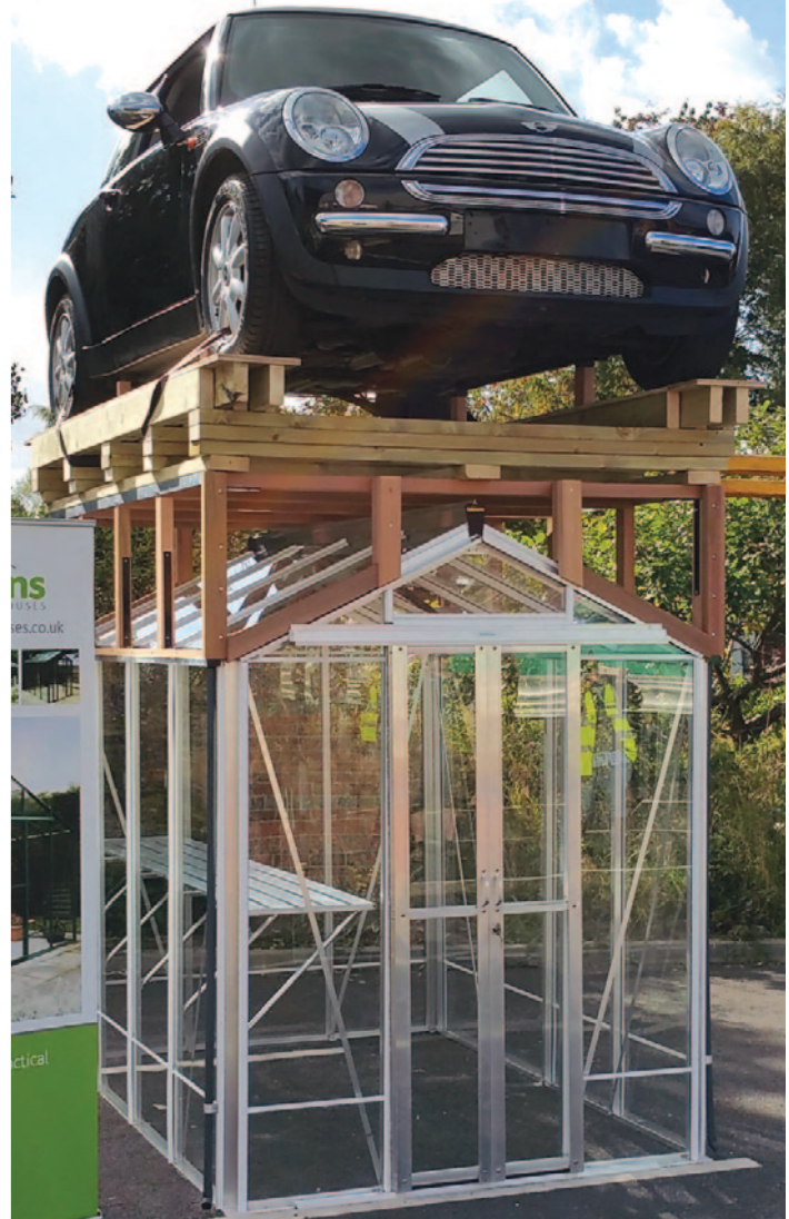
This amazing demonstration of strength took place in September 2015. Although a special frame to level the roof was made, the greenhouse underneath was completely standard and unmodified! The mini weighs nearly 1.5 Tonnes.
